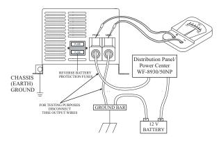
If the converter output voltage reads in the 13.6 Vdc range and the battery is not charging, check for:
