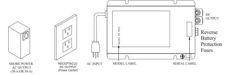
If the reverse polarity fuses are blown, it means the RV battery was accidentally connected in reverse, either at the battery or at the converter. Reconnect properly, then replace the fuse with the same type and amp rating as the original "Littelfuse" Type 257 automotive-style fuse.
